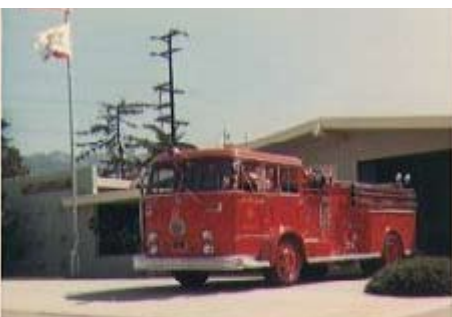
Engine 82, a 1963 Crown, was one of the first four-door closed cab rigs used by LA County Fire, and it was the first of the department's engines to be equipped with an automatic transmission.
