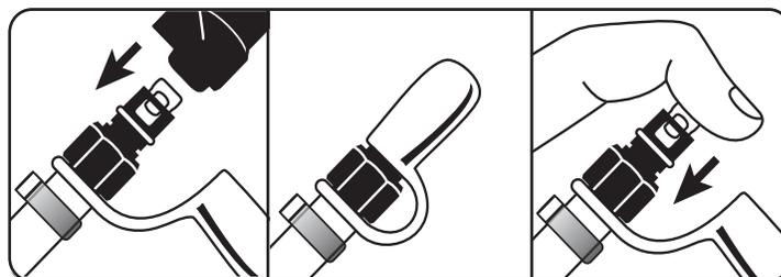
10. To prevent accidental valve opening, whenever a patient is being moved in the mattress or when the mattress is being put away, make sure to **ALWAYS** place the RED LEASHED CAP over the end of the MaxiValve™ .
